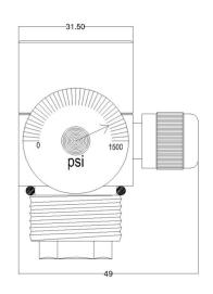
The Integrated C10 Valve is a combination of a C10 valve and a single stage pressure reducing design. This product can be directly connected to a 17L and 34L cylinders.
