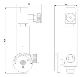
The Septum Regulator is a special regulator intended for laboratory gas applications in which a syringe is used for extracting the gas sample.
