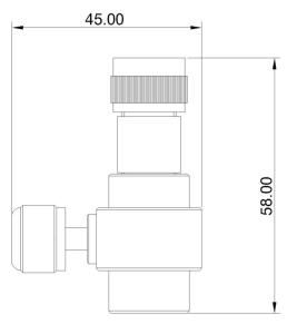
The Septum Valve With Aerosol is a special regulator intended for low pressure laboratory gas applications in which a syringe is used for extracting the gas sample.
