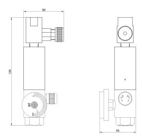
The HP Septum Regulator is a special regulator intended for laboratory gas applications in which a syringe is used for extracting the gas sample.
