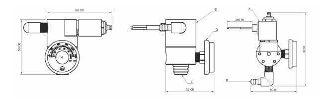
The solenoid regulators are solenoid operated and used with dry gas compact machines.
